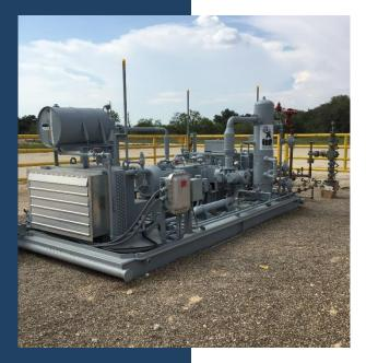
With the reliable Ariel® compressor frame at its heart, every other component of the old school gas compressor package has been redesigned for compressing rich gas at the wellhead.
