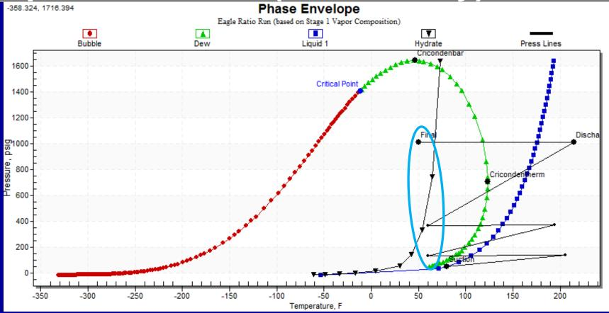
Temps fall below 120 F, allowing SIGNIFICANT hydrocarbon condensation since gas is richer
