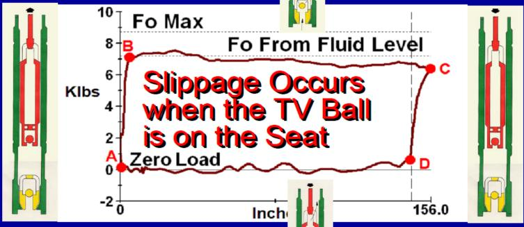
4) Point D to A, TV open as fluid in the pump is displaced through the traveling valve on the down stroke
