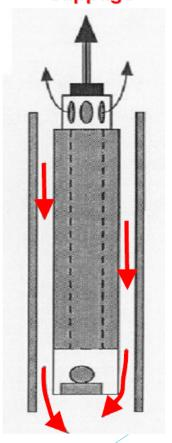
1) Point A to B pressure acting on closed SV gradually transferred from tubing at point A to be fully carried by the Closed TV at point B.
